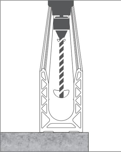
1 - Drill the support with a tool adapted to it.
