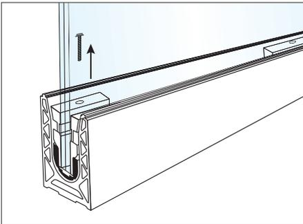
3 - Finish unscrewing the screw and remove it
