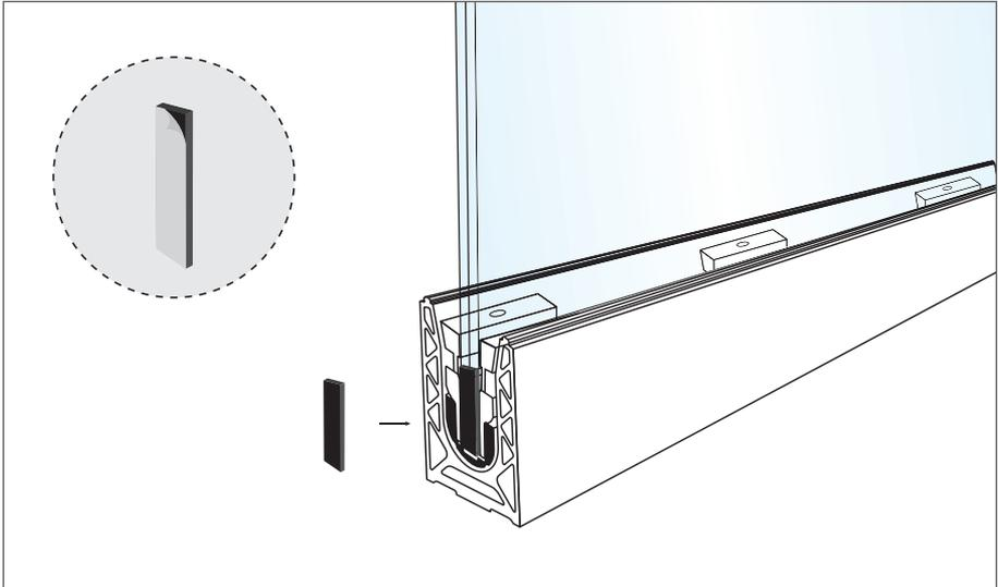
1 - Remove the protection from the adhesive. Stick the SADEV spacer on the edge of the glass, on the bottom right-hand corner flush with the glass.
