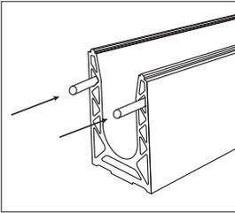
1 - Fit 2 SADEV pins connector in the rail section holes.
