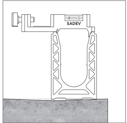
2 - Clip the specific levels on the profile, at a useful distance to put your level (see top view).
