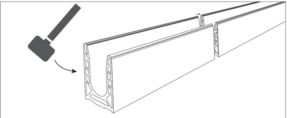
2 - Connect the rails together by using a mallet.
