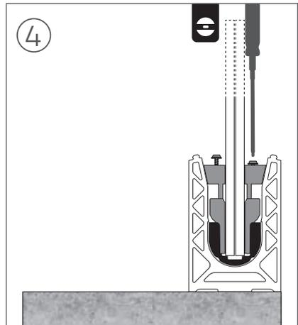
1 - Screw on each side of the glass as long as you do not change the level of the glass.
