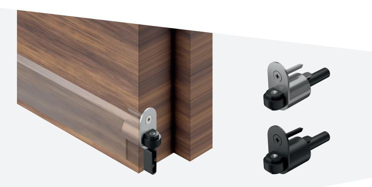
The rotating activator of the trigger module enables the application range of Planet US for pivot doors to be extended. Thanks to the power absorption via module, the seal maintains its long service life and requires only minimal triggering forces. The module is available in black and stainless steel to suit any door design.
